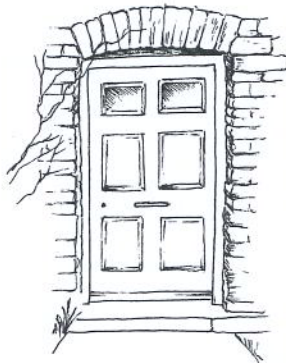
Fig. 17 Typical farmhouse doorway with segmental stone arch
