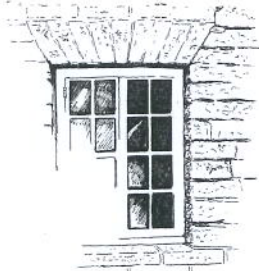
Fig. 15 Flat arch with wedge shaped stone voussoirs
